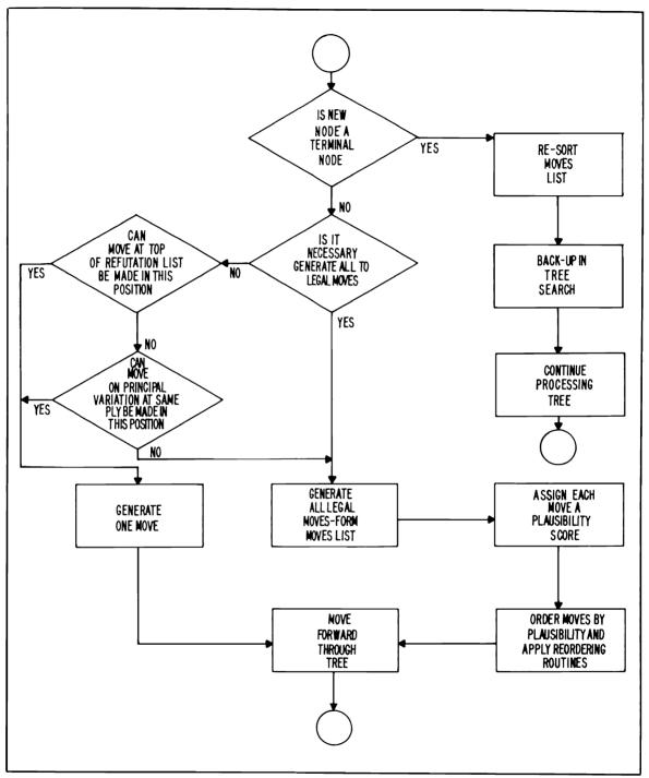
Fig. 7-17. A flowchart for node processing.
